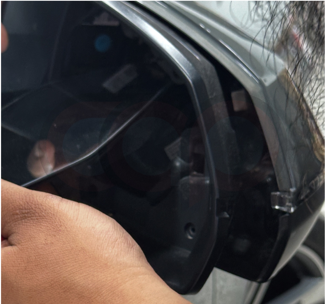
Image 5: Removal of Mirror Housing Cover
