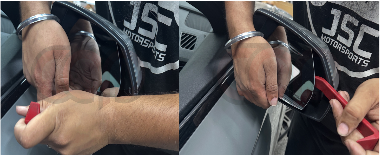
Image 1: Prying out the mirror from underneath
