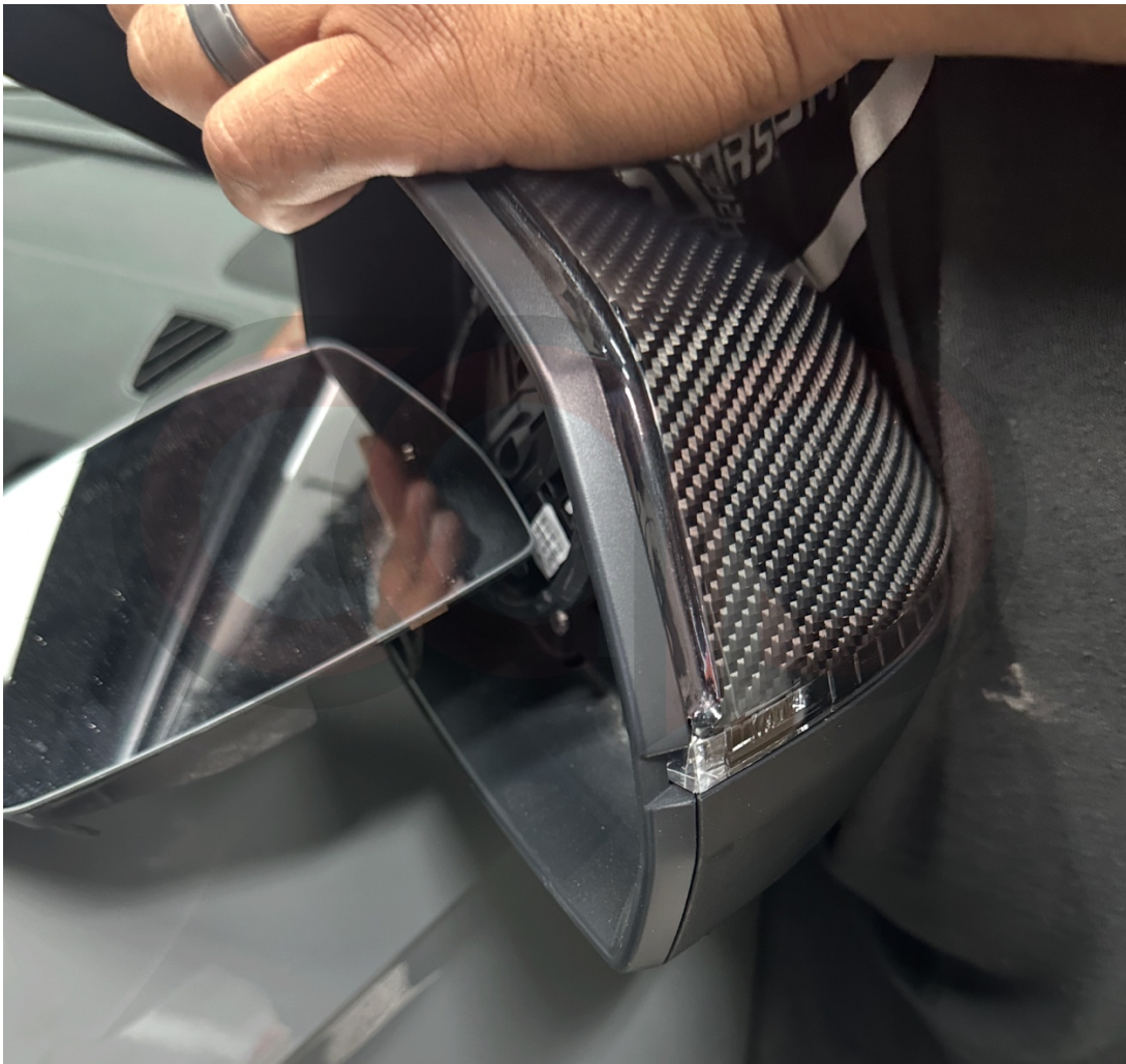
Image 10: Attach Mirror Housing Cover
