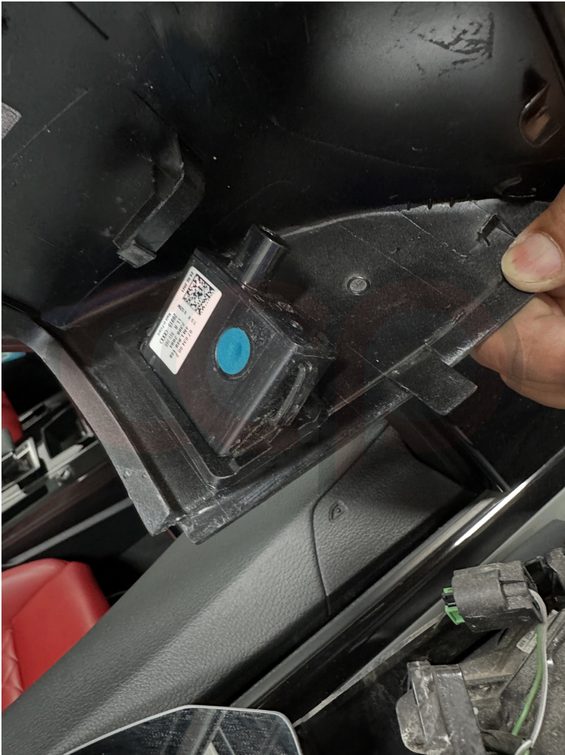
Image 9: Disconnecting Lane Assist Module
