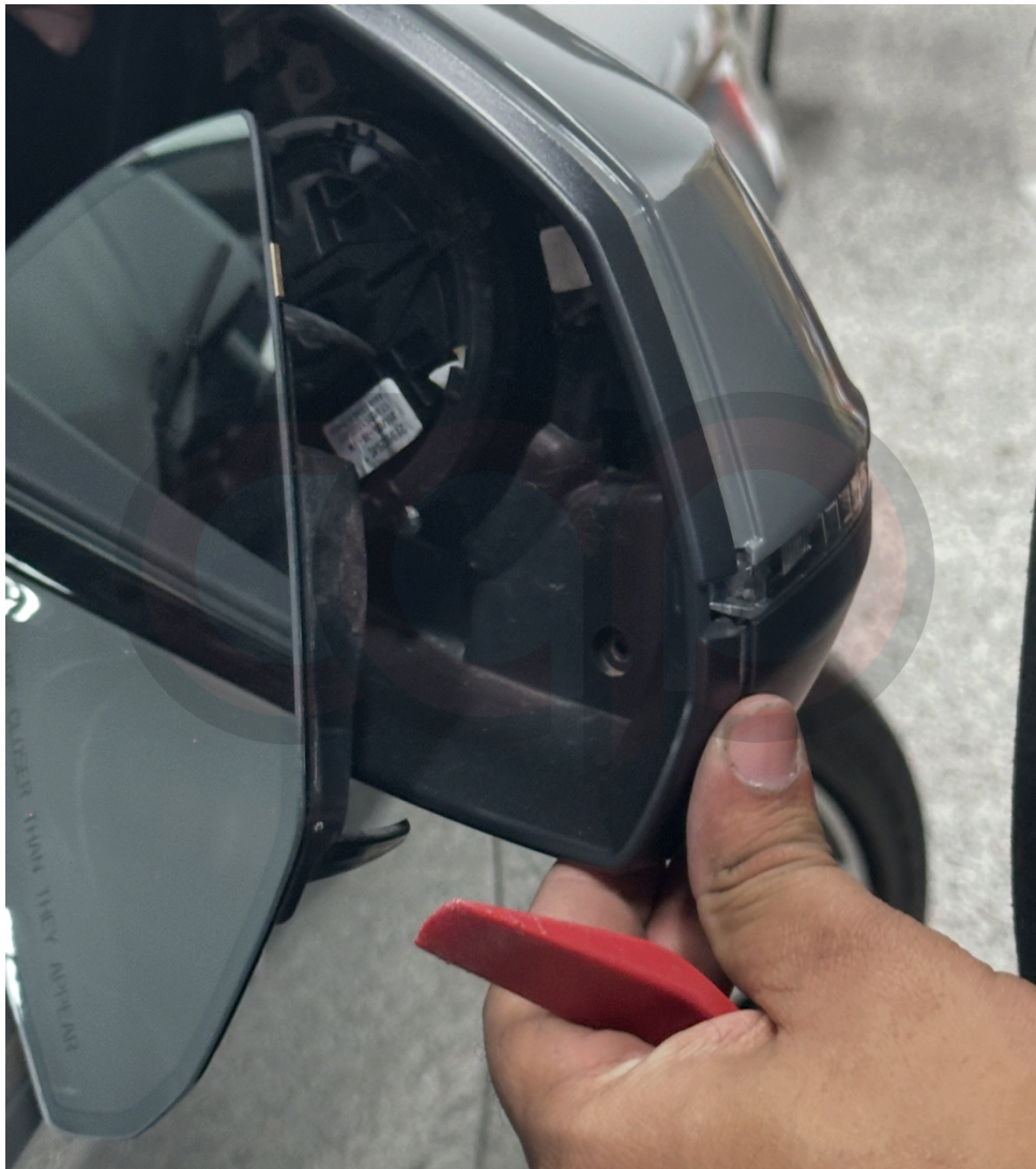
Image 4: Removal of Mirror Housing Cover
