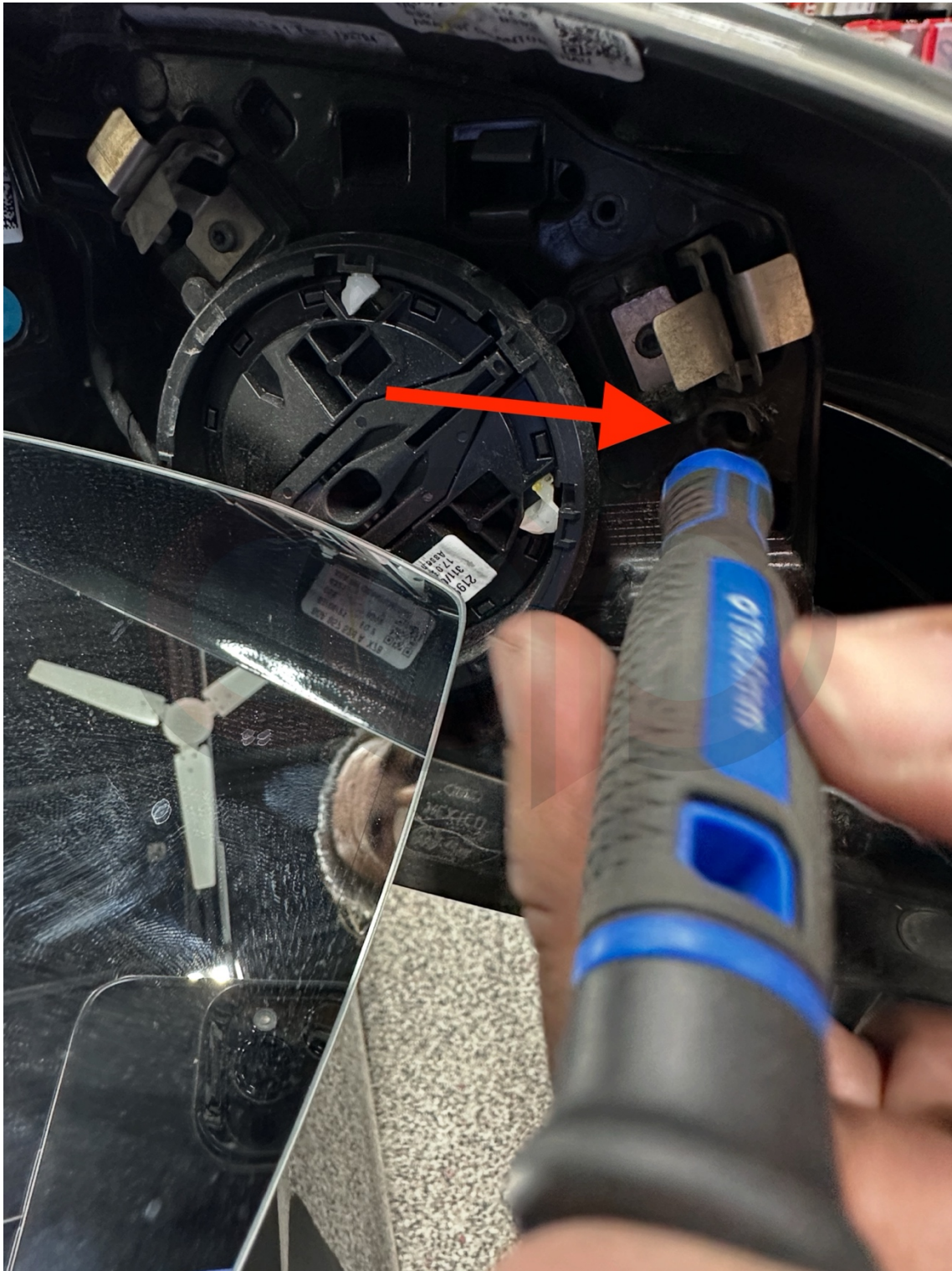
Image 6: Location of T10 Screw holding Mirror Cover
