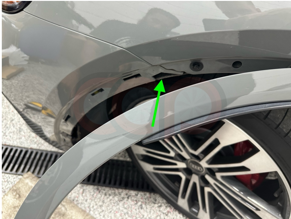
Image 7: T25 Screw hidden underneath the corner of the bumper
