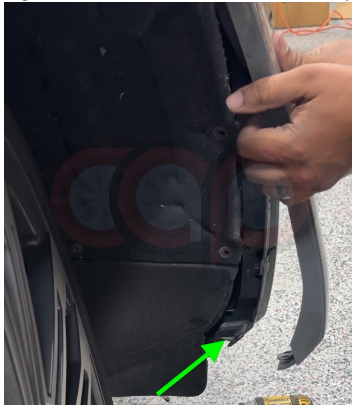
Image 5: T25 Screws underneath the bumper and removal of trim piece
