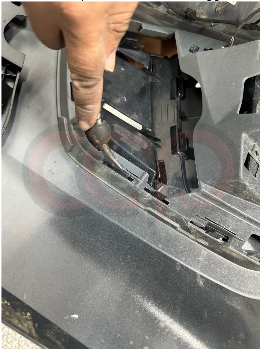
Image 16: Disconnecting tabs from the bumper
