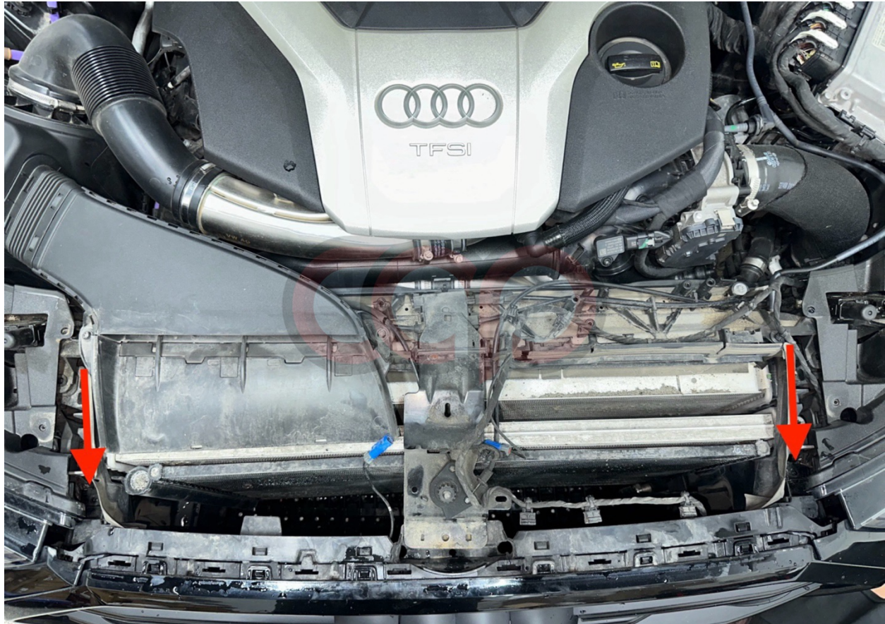
Image 6: T25 Screw removal positions.
