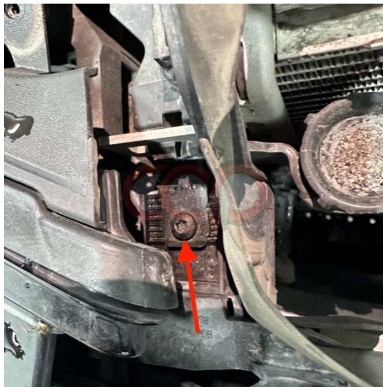
Image 8: T25 Screw close up left side
