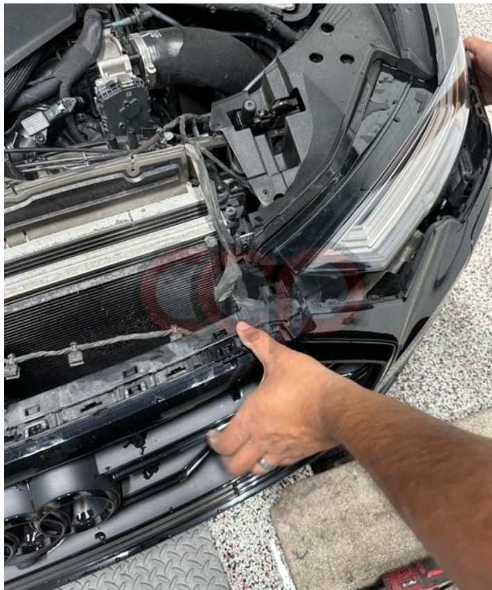
Image 12: Driver Side Bumper removal
