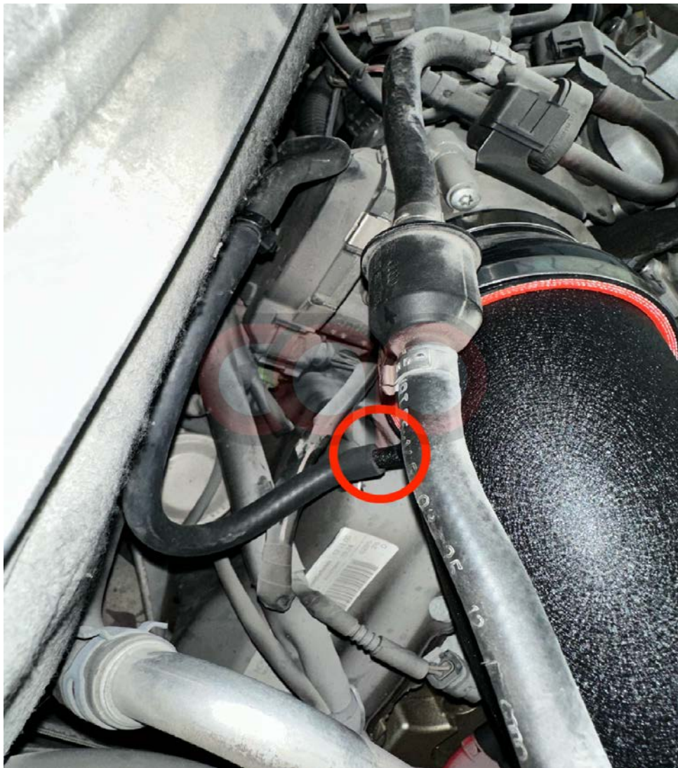
Image 12: Attaching Vacuum Hose to Intake Pipe
