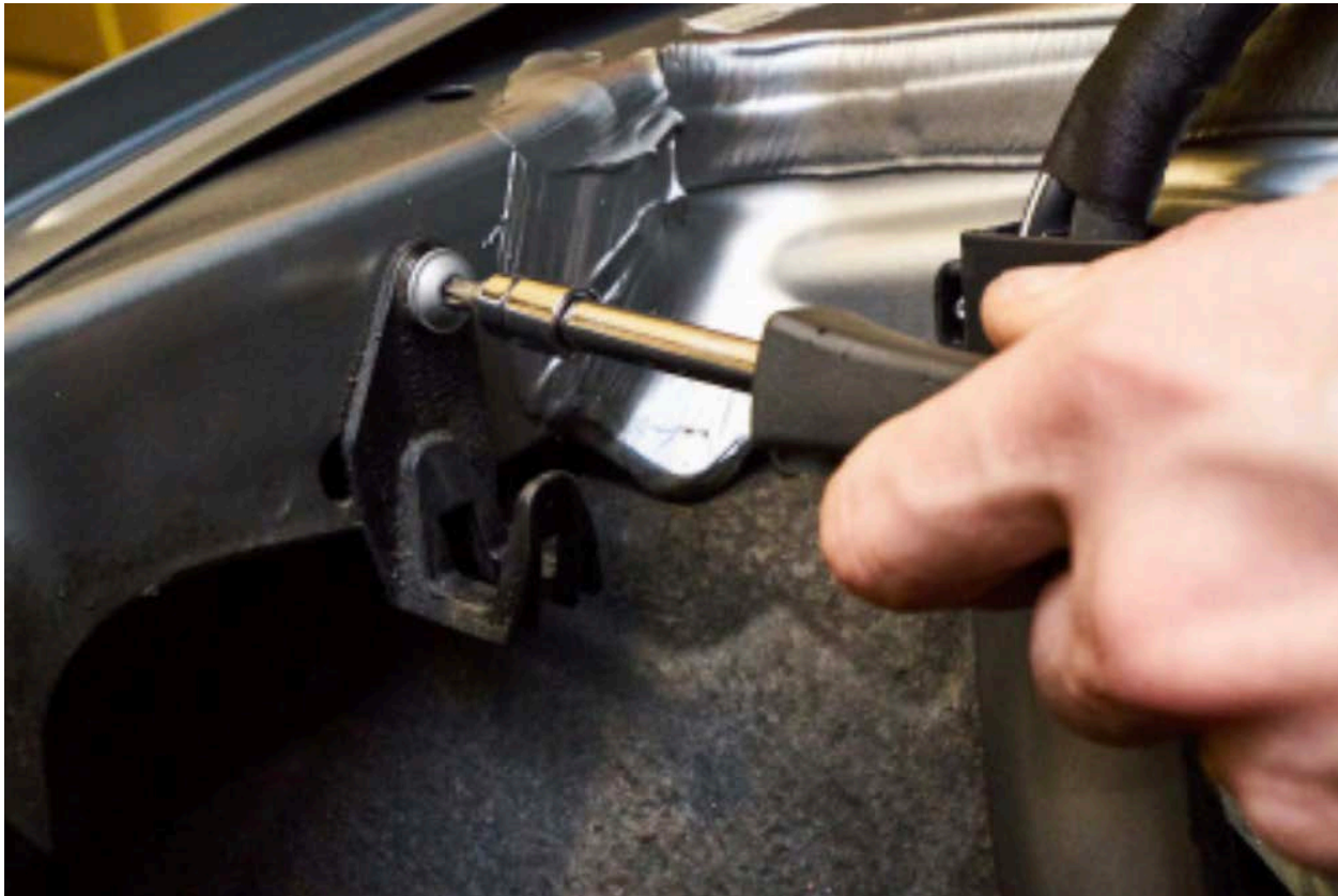
Image 6: Removal of factory airbox mount
