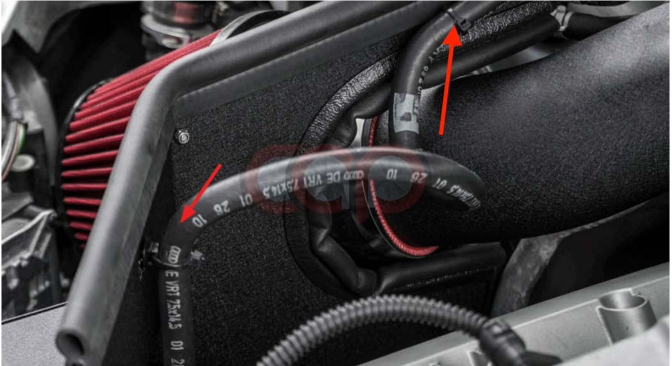
Image 13: Securing Fuel Return Lines
