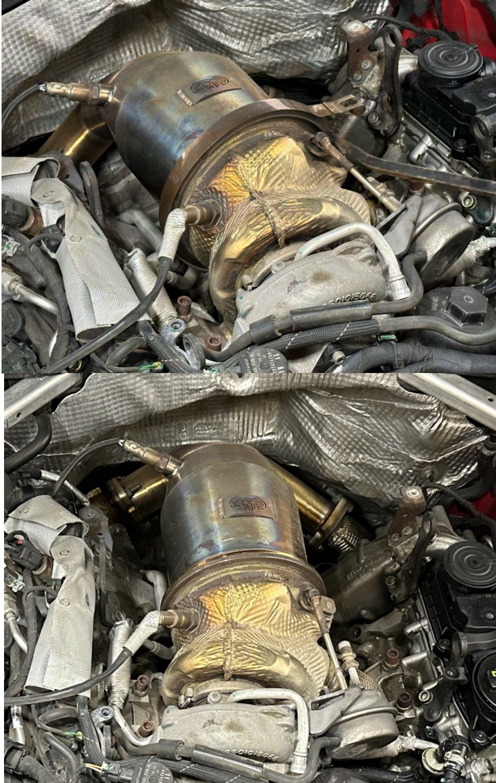
V Band Clamp removed from the stock downpipe
