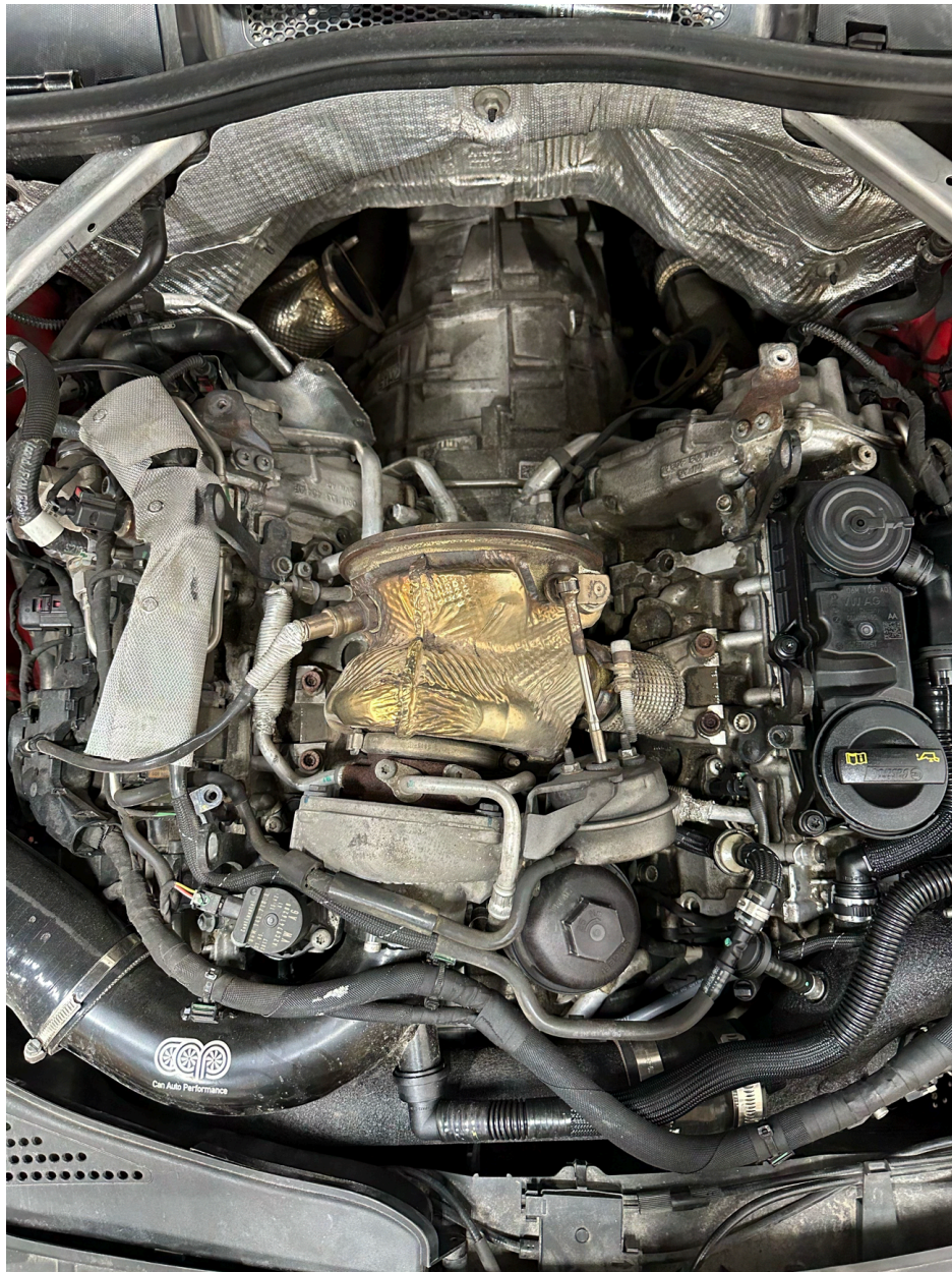
Stock downpipe removed from the engine bay
