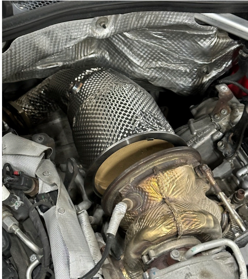
CAP downpipe being placed into the engine bay
